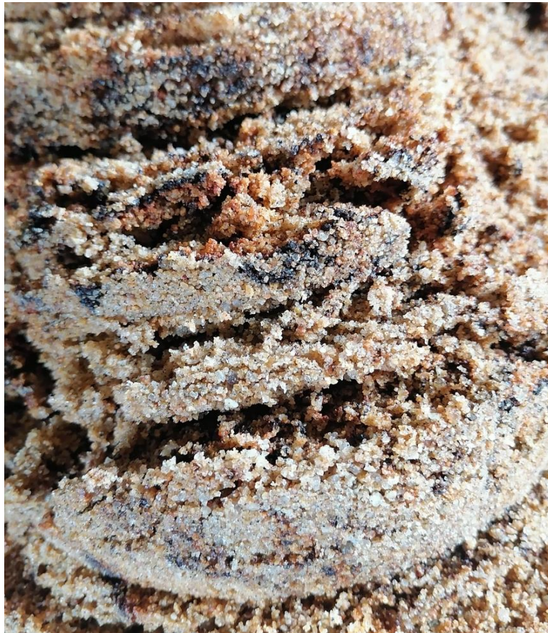
Picture of cake formed in the filter during the elapsed time of 1 year.
