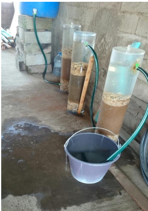
Figure 4: Picture of the designed filtration system: Well water was stored in blue 200 L tank. The first and the third columns are conventional bio sand filters (BSF). In the middle of column 2 is Fe 0 SW mixed with sand coarse (Picture B). The columns are connected to each other with a PET tube.
