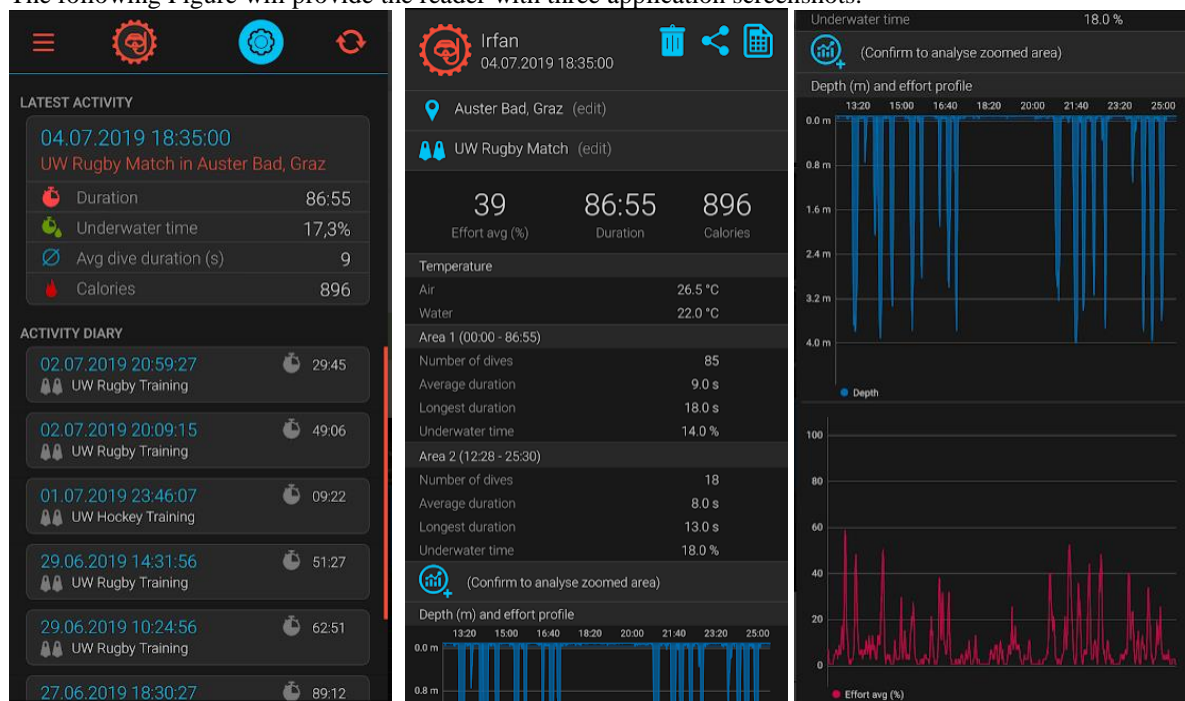
Fig.3. pete3d Android application screenshots. The first on the left shows a list of dive logs. The middle screenshot provides the metadata of one of the dive logs. Besides, it provides a statistical analysis of a selected dive log part. The screenshot on the right provides the visualisation of the depth, and the “effort” – which is a part of an ongoing research.
