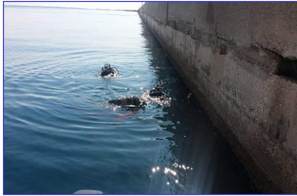
Fig.10. N.3 ESDs during the sampling phases of scraping on an artificial jetty
