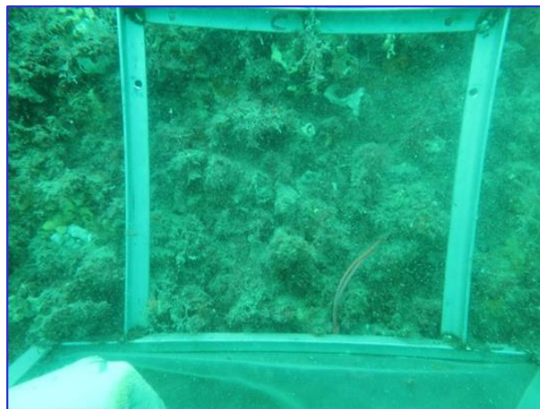
Fig.11. The metal square 32x32cm used by ESDs during the scientific diving
