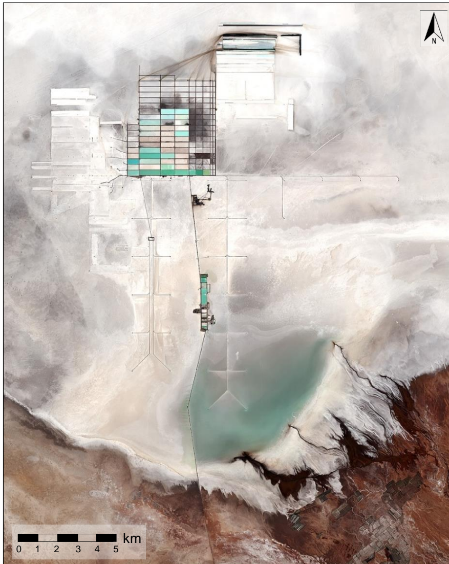
Fig. 61: System of evaporation pans near the Río Grande delta for the extraction of elements from the brine by the national mining corporation Comibol (image taken by the Copernicus Sentinel- 2B satellite on 17 May 2017 and provided by ESA 1 )
