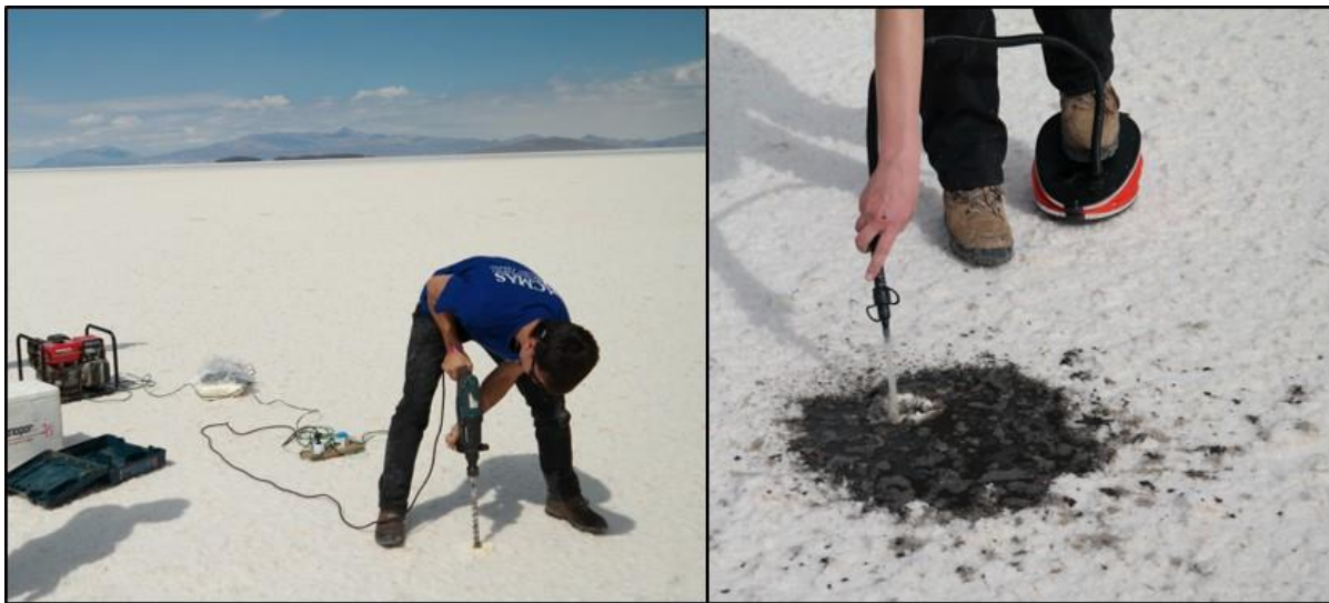
Fig. 16: Auger drillings with a Bosch drill hammer (left) and using air lift for cleaning the bore hole from drill sludge
