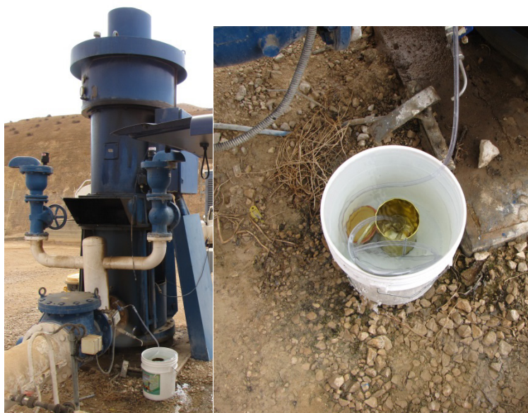
Figure 6 Sampling of CFCs and \text{SF}_6 from well pump; left: well pump and 10l container for sampling, right: 10l container with glass bottle and tin connected with a tube to the pump during flushing with water
