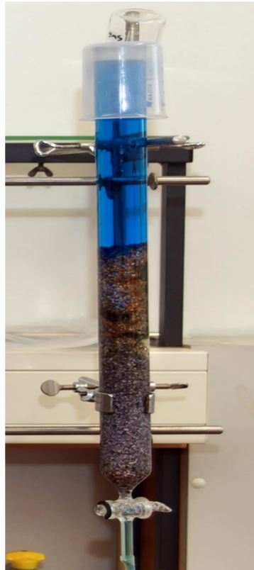
Figure 16. Brown discoloration within and surrounding the reactive zone indicate that iron corrosion products formed and were precipitated. The blue solution within the column is Methylene Blue, which was added at the end of the experiment as part of a subsequent experiment not included in the present work.
