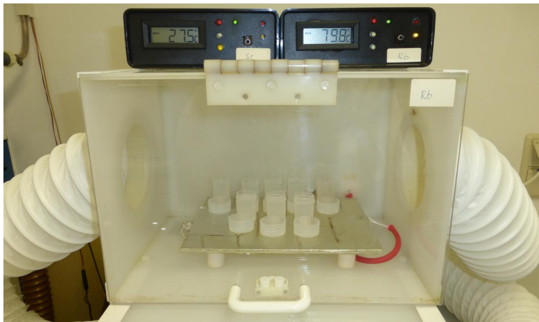
Figure 15: Clean oven for drying water samples at the Isotope Geochemistry and Geochronology Laboratory at the Mineralogy Department of the Technical University Bergakademie Freiberg, Germany.
