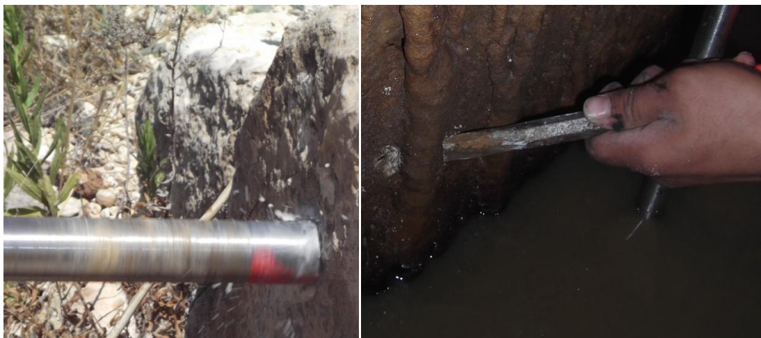
Figure 16: Sampling methods using: left a core drill and right a chisel
