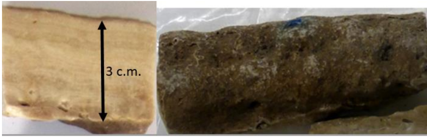
Figure 71: Sample A-1(a) cross section shows the lamination and outer side of the sample
