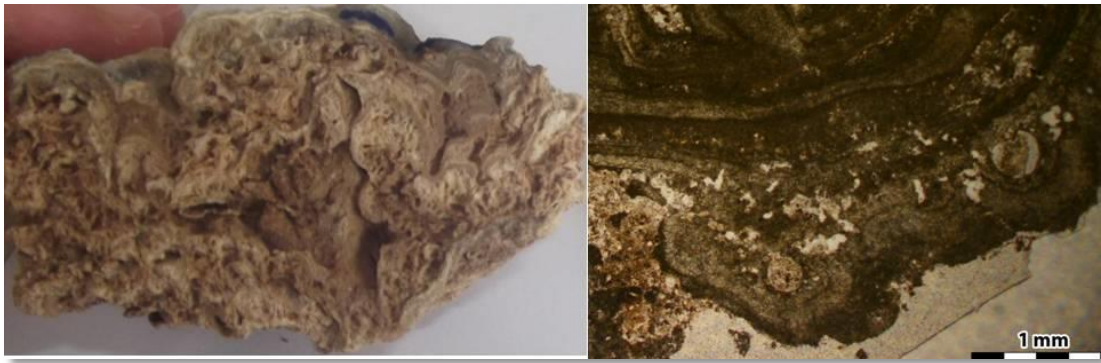
Figure 104: Sample A-6, left: cross section of sample, right: thin section shows lamination
