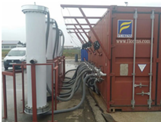
Fig. 1: Rock filled cylinders for the flow-through experiments with CO 2 impregnated water
