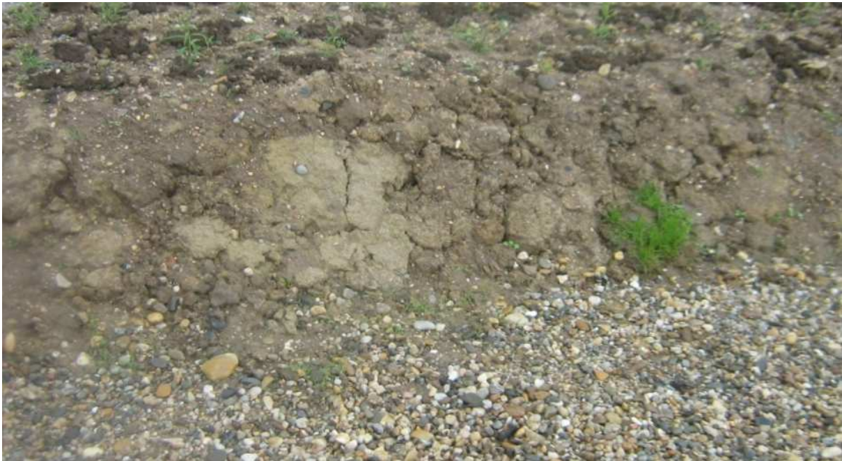
Fig. 2: Soil formation on a gravel layer (simulation of a layer with suspended capillarity)
