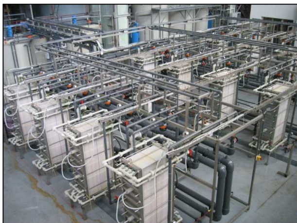
Fig. 4: Industrial electro dialysis in ZSNP plant
