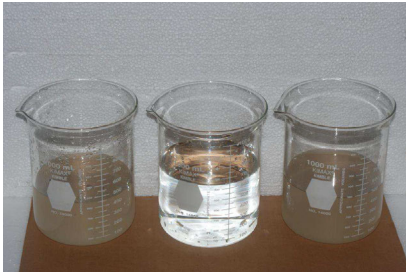
Fig. 5: Samples from filtered PW with a 0,9 nm pore size ceramic nanofiltration membrane ( From left to right: Feed, permeate, concentrate) (Nijmeijer 2014).
