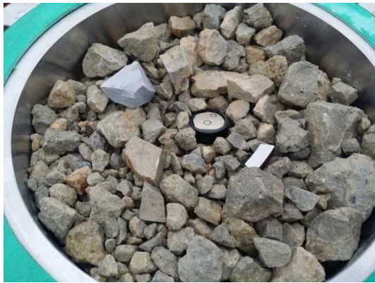
Fig. 2: Steel, concrete and polished rock samples in the rock cylinders
