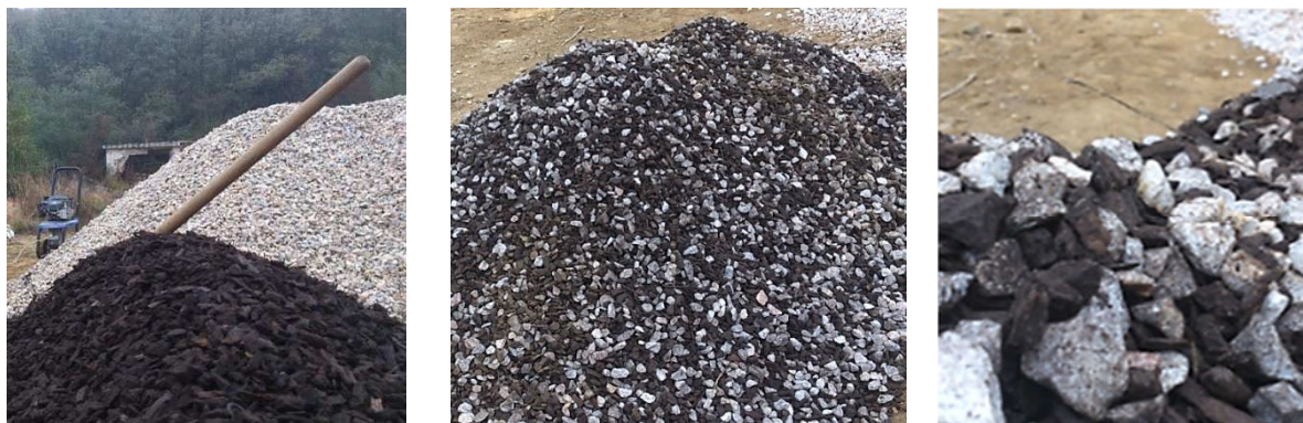
Fig. 7: Materials used in the passive AMD treatment pilot test (a (both pictures on the left side), grounded limestone and grounded lignite; b (right picture), mixture of the grounded materials)
