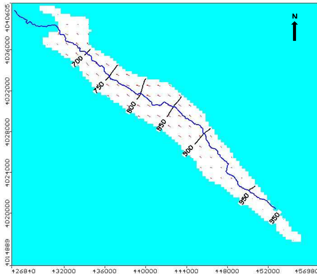
Fig. 8: Groundwater head equipotential (black line) and flow directions (red arrows) in Mirawa valley, contour interval is 40 m, UTM WGS-84 coordination system
