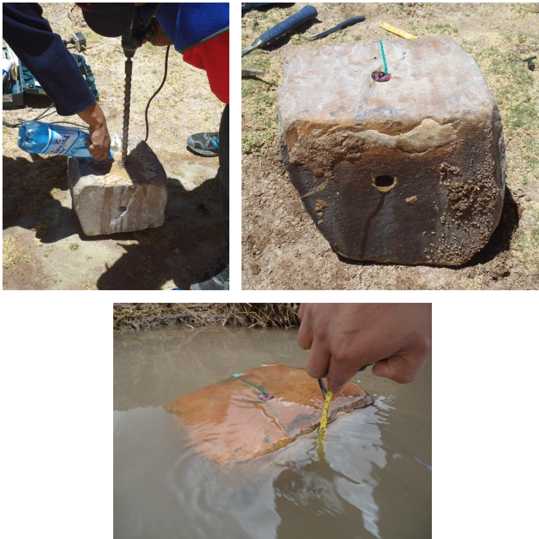
Figure 17: Preparation of a boulder for the installation of the CTD-Diver in the Rio Grande for long-term monitoring of the river level.
