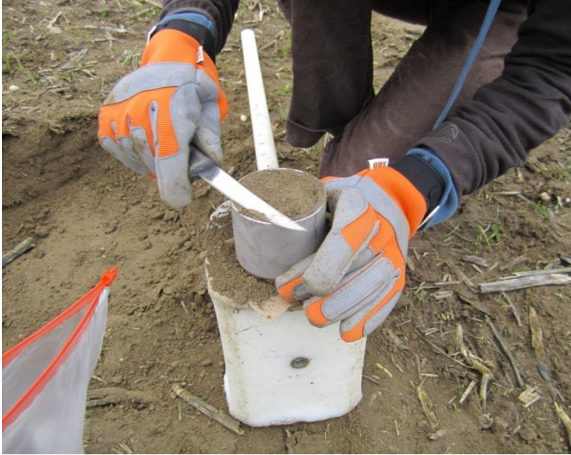
Figure 6 – Leveling top and bottom of a sample from 12 cm depth enclosed in liners and metal core cutter
