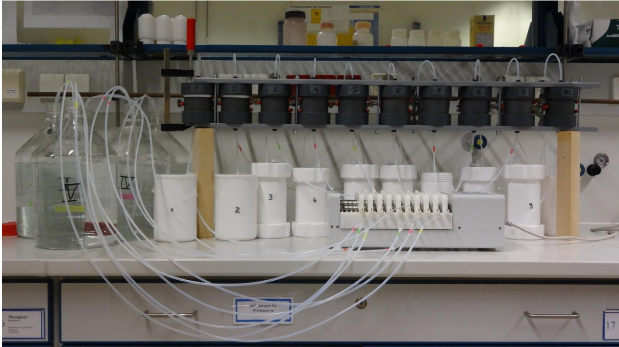
Figure 8 – Setup for flow-through experiments (left side of the picture: 5 L storage glass bottles (labeled with I to V), upper part of picture: dark grey PVC flow-through cells (labeled with 1 to 10, 1-5 being from upper soil level, 6-10 from lower soil sampling level), below: white Teflon collecting vessels (labeled with 1 to 10 according to corresponding flow-through cell), in foreground: peristaltic pump with pumping tubes and hose connectors. Teflon tubes throughout the system for connecting the individual units.)
