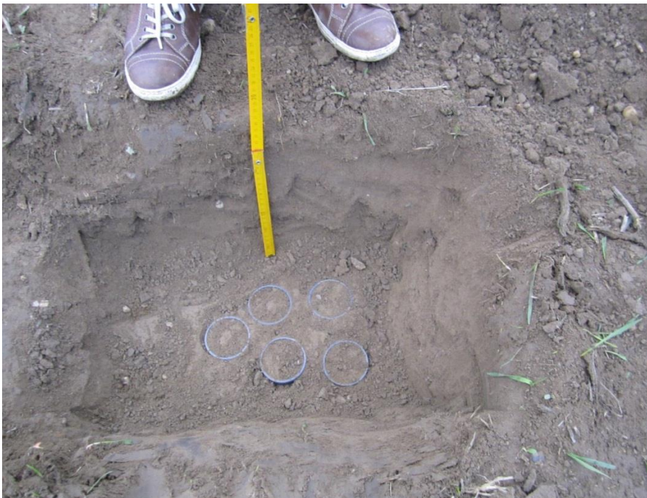
Figure 5 – Undisturbed soil sampling at about 26 cm depth using only PVC liners without steel core cutters
