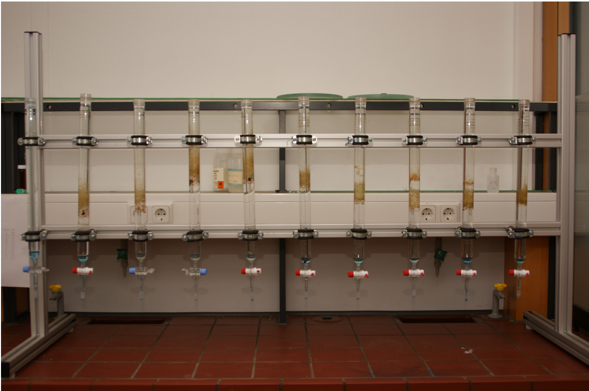
Fig.6: Visual appearance of empty columns after disassembling of packed materials from columns.
