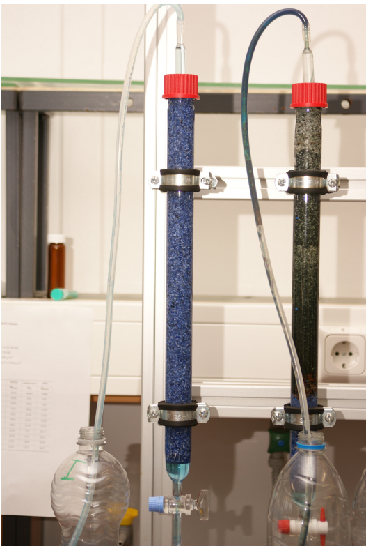
Fig.4: Different coloration patterns of columns at 131 th day: (a) uniform coloration of sand column (column 1), (b) non- uniform coloration of Fe 0 +sand columns (column6,7 and 8).
