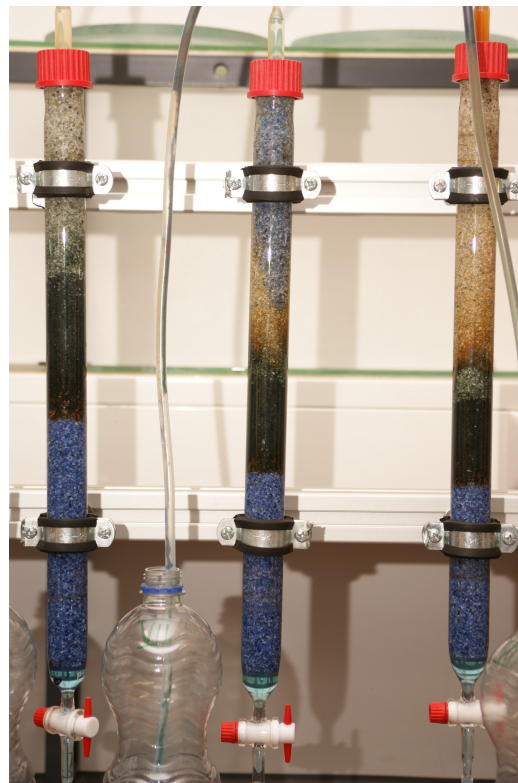
Fig.4: Different coloration patterns of columns at 131 th day: (a) uniform coloration of sand column (column 1), (b) non- uniform coloration of Fe 0 +sand columns (column6,7 and 8).
