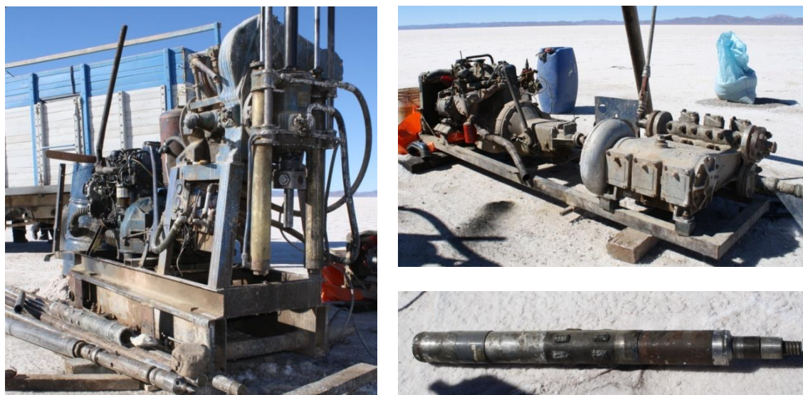
Fig. 7: Drilling machine of the Bolivian drilling company (left), pump for drilling fluid (top right), core barrel for cores with a length of 1 m and a diameter of 4" (down right)
