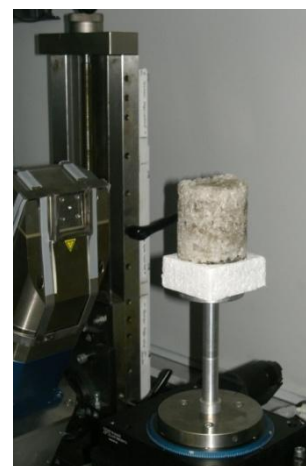
Fig. 14: Fixation of the core sample in the instrument
