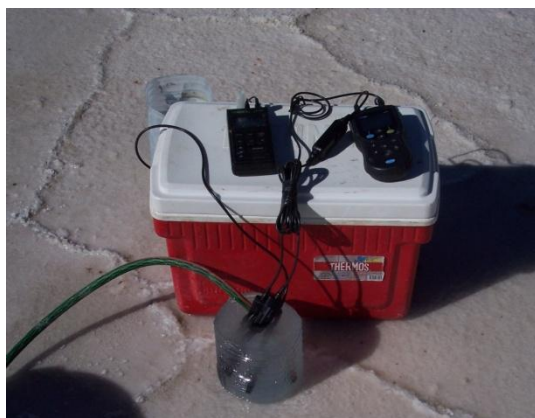
Fig. 13: Determination of field parameters of the brine in a flow through cell
