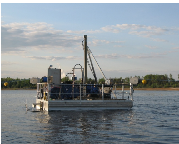
Fig. 1: Base of the pilot experiment in lake Burghammer: Floating platform, CO 2 injection technology.
