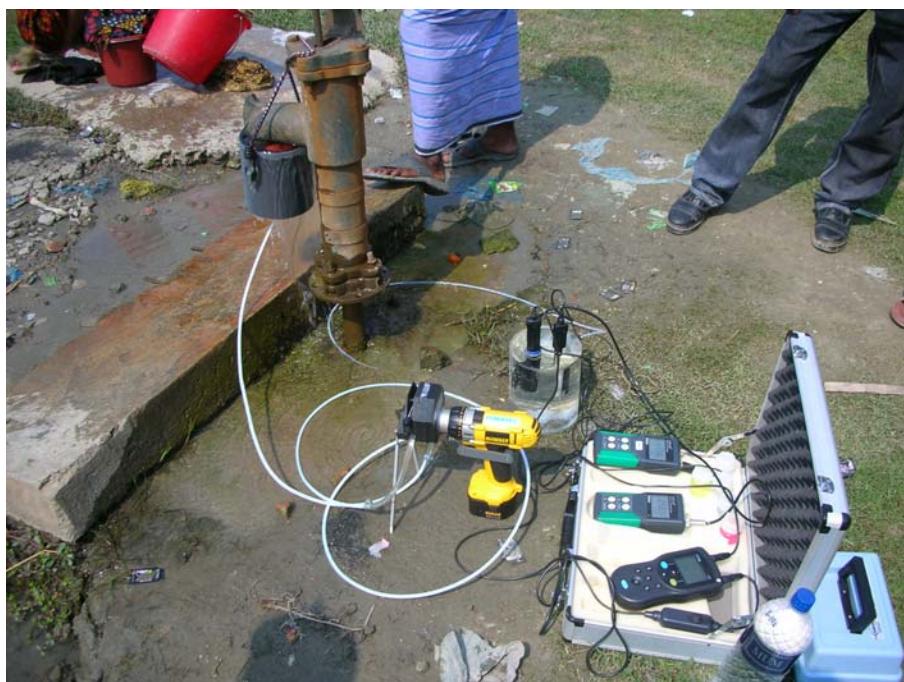
Fig. 4.1.2.1. Sampling procedure for village wells by connection of a bucket (to avoid oxygen contamination and to connect the Hand-pump NO.5 with the transportable pump)
