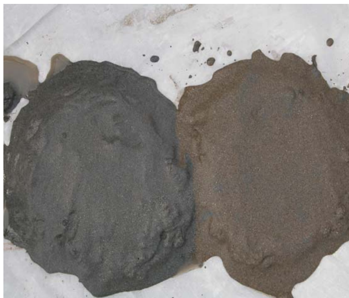
Figure 5.1.1 Reduced sediment from the shallow aquifer on the left and oxidized sand from the deeper aquifer on the right.
