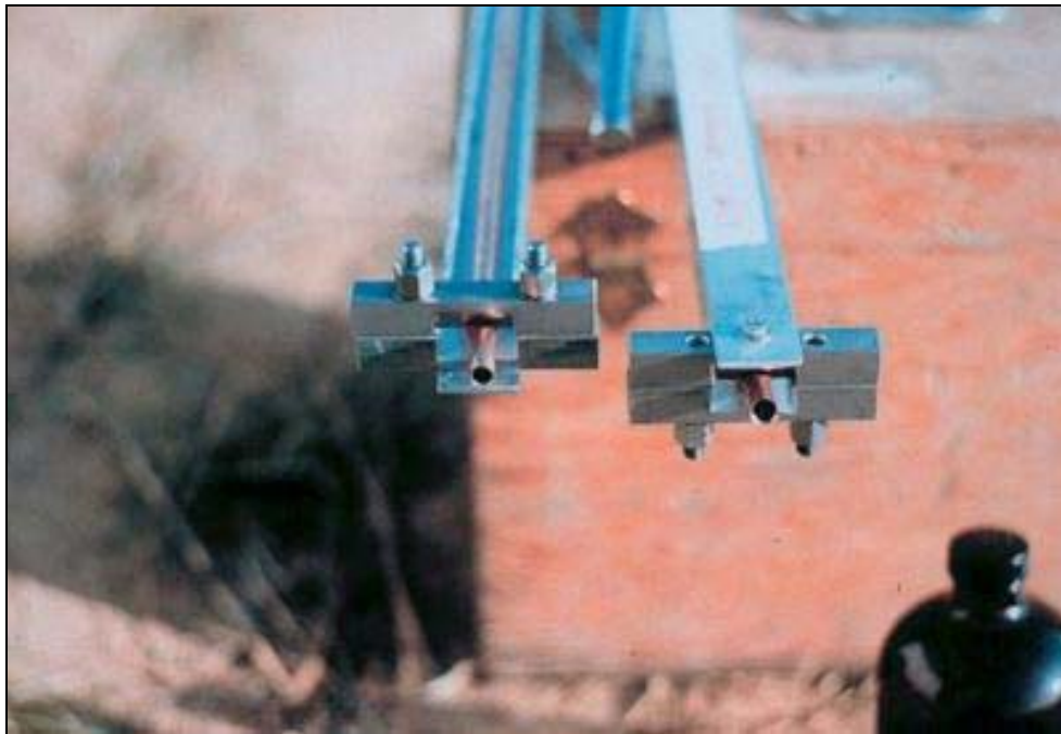
Fig. 2.6: Properly cold welded copper tube.
